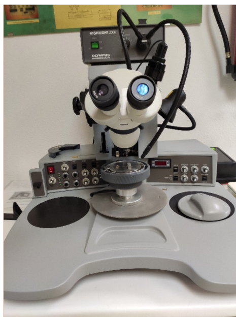
Figure 23. RF Facilities. Wire & ribbon bonding. Kulicke&Soffa 4526.
