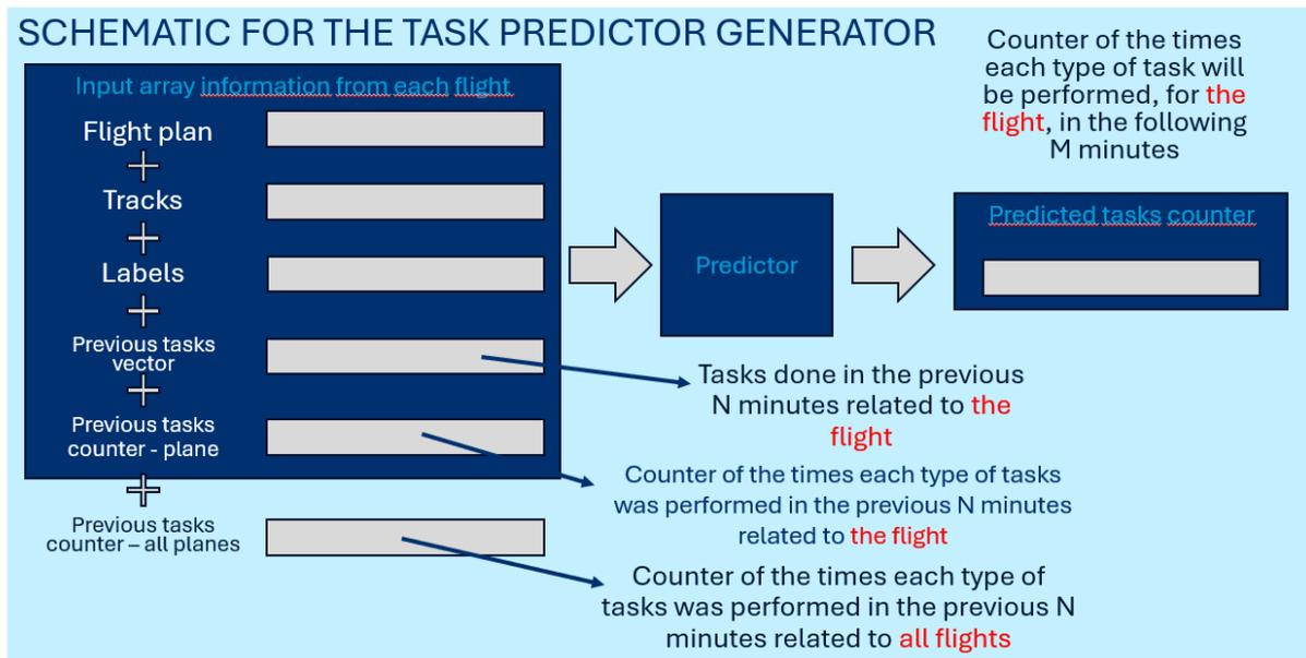
**Figure 10:** Task prediction generator inputs and outputs schema
