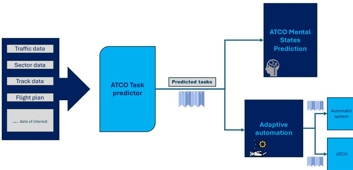
Figure 1: Potential ATCO task predictor roles in CODA architecture
